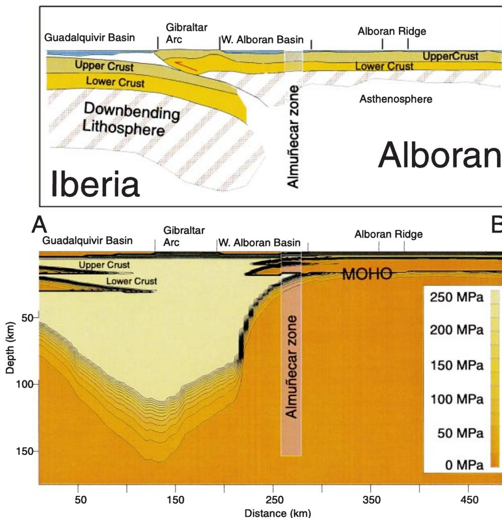
**Fig. 4** Bottom: integrated compressional strength along profile A–B (Fig. 2F) showing dramatic increase of crustal strength over the Almuñecar zone. Top: schematic interpretation. See Tables 1 and 2 for the input parameters used in the calculations. Crustal thickness is constrained by seismic reflection and refraction data.
